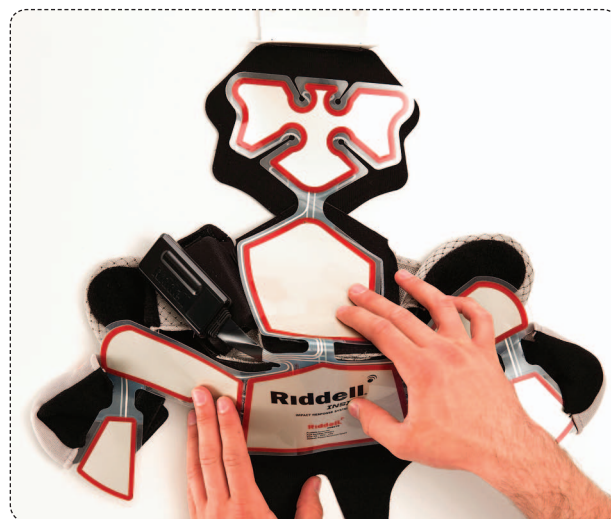
FIGURE 2 Developed by researchers at the Ohio-based company Simbex, the technology behind the InSite system includes an electret film within the helmet’s liner assembly. The electret film allows the system to run on a single battery for an entire season. (Photo courtesy of Riddell Sports, Inc.)
